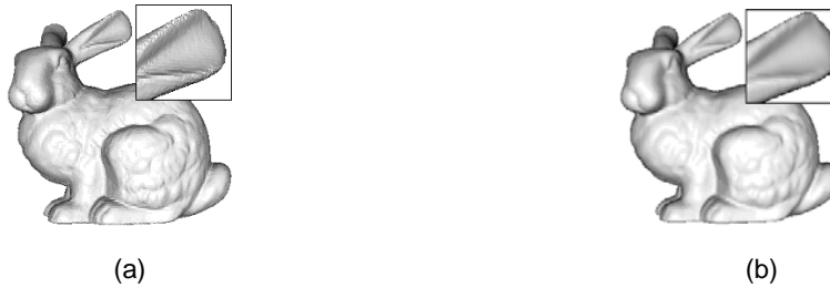
Figure 3. (a) The original “Stanford Bunny” model (69451 polygons). (b) Smoothed model after one iteration based on 11-point interpolation. Processing time: 4.7 sec.
